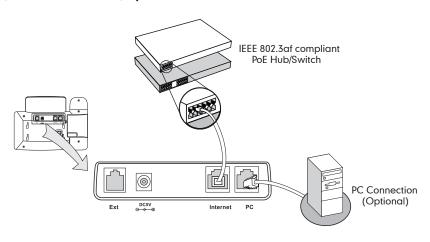
**Note:** If inline power (PoE) is provided, you don't need to connect the power adapter. Make sure the Ethernet cable and hub/switch are PoE compliant.
